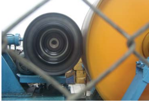
Tyron ATR undergoing load and speed testing
