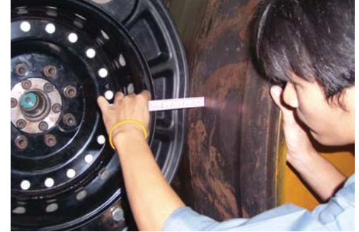
Measuring unique load deflection characteristics
