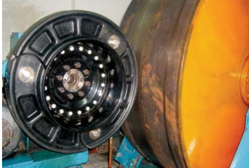
Setting up Tyron ATR for testing on a rolling road
